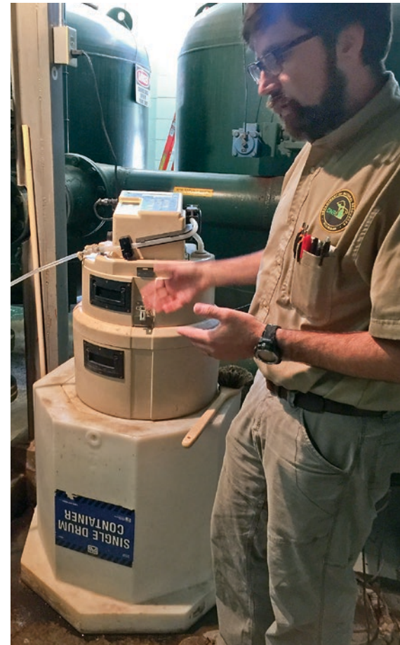
Above: Paul Stowe explains how an automatic water sampler grabs a 60 ml sample every half hour at six different points in the hatchery process.
