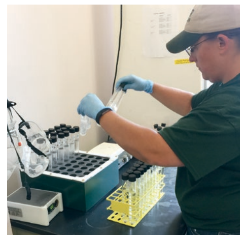
Photos: Top, on the lake, the tube sampler enables a grab sample at specific depths. Second, reagents are added to each sample. Third, Samples are placed in the digester. Bottom, The spectrophotometer reads the color density to calculate phosphorus concentration.
