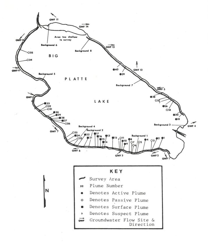
Figure 3. Location of the septic leachate survey area, plume sites, and groundwater flow monitoring results on Big Platte Lake, Benzie County, Michigan.
