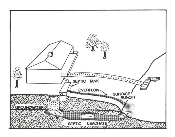
Figure 2. Types of septic system failures likely to cause contamination of groundwater and surface waters
